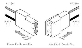
MOLEX Series 1545 connector for use in promoting compatibility and interchangeability among personal VHF/UHF radio equipment at disaster sites. Polarity should always be verified prior to connecting to radios and power supplies.
